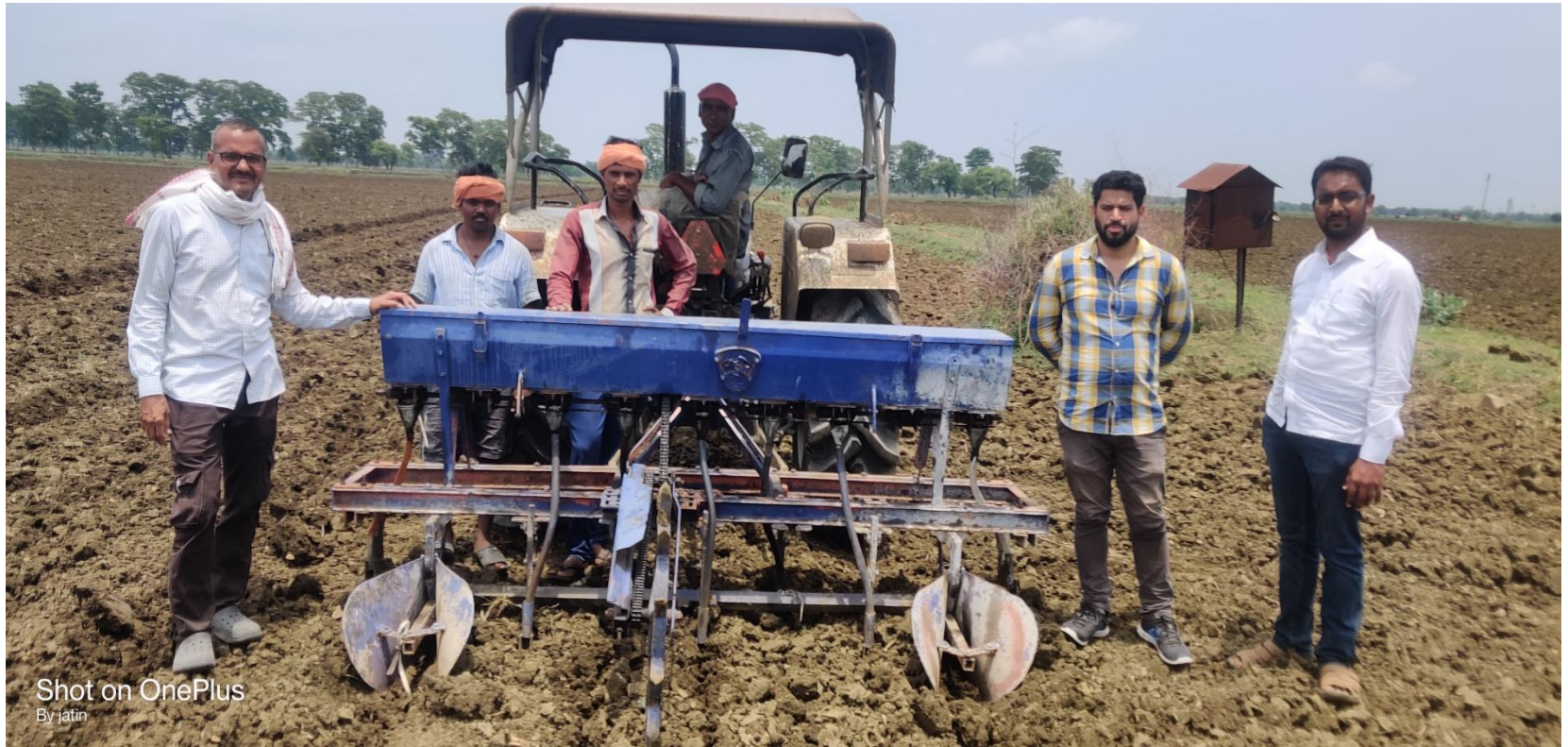
Broad bed cum intercropping sowing machine for Soybean-pigeonpea
